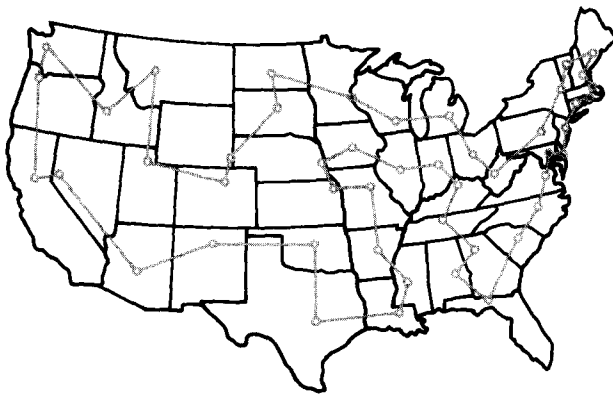
Figure 10.3: By traveling this route, a salesman could visit all forty-eight state capitals and clock the lowest possible mileage.
